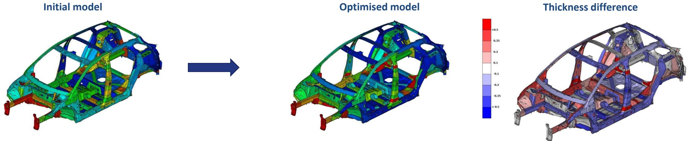
Example : optimization of the Peugeot 3008 to minimize the vehicle weight while satisfying the norms for chock resistance.
