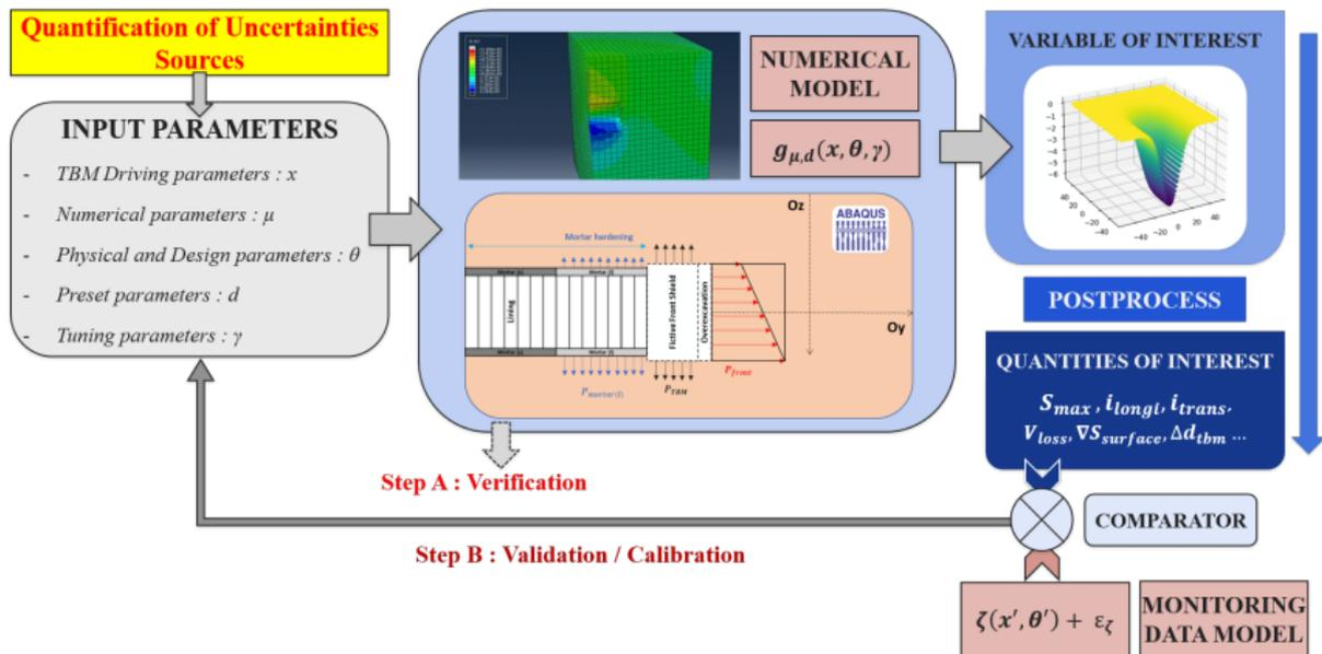
**Figure:** Objective of TBM Excavation Simulator Calibration [2]
