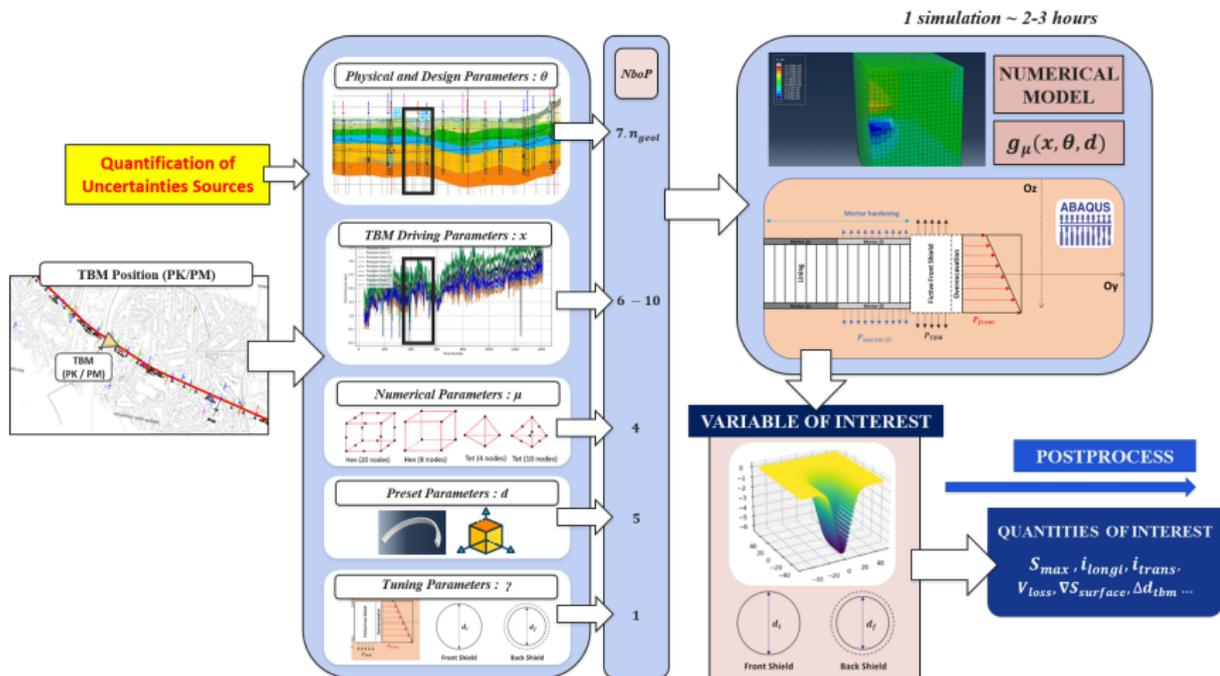
Figure: 3D Parametric Finite Element Model of EPB TBM Excavation[2][6][9]
