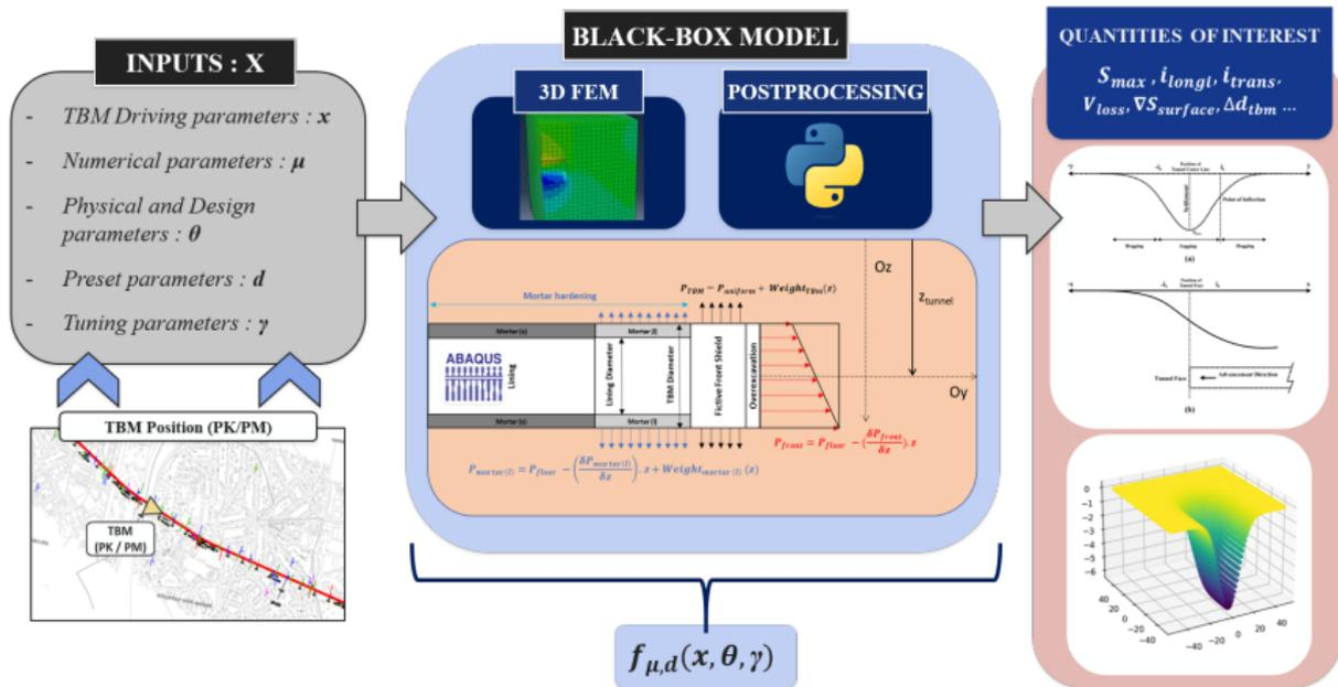
**Figure:** Modeling the TBM Excavation Simulator using a BlackBox approach
