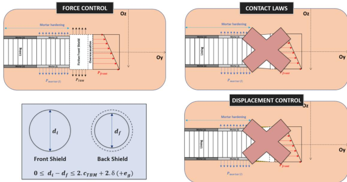
**Figure:** Different Strategies to model TBM excavation [5]
