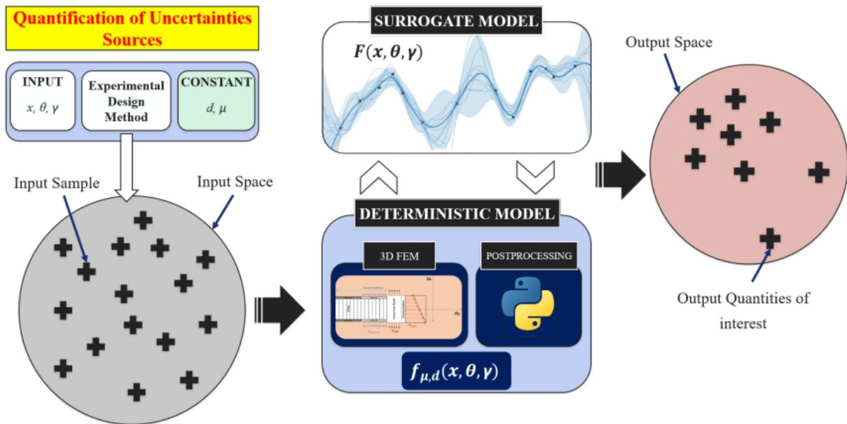
**Figure:** Surrogate Model of the TBM Excavation Simulator [2]
