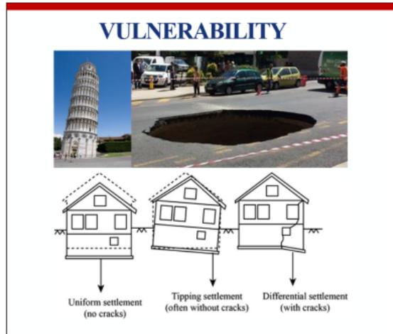
**Figure:** Surface Settlements (left) and "Fontis" observed during tramway construction in Nice (left)
