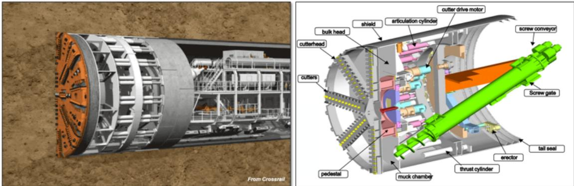
**Figure:** Tunnel Boring Machine - Earth Pressure Balance Technology
