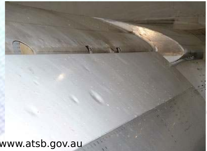
Hail damage on B767 slat
