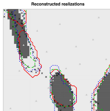
Figure 2: GRF model for the negative Branin-Hoo function with 20 evaluation points (gray triangles). 3 realizations of the random set are generated by simulating at 100 optimally-chosen points (black crosses) and predicting the field at the 50 \times 50 grid.
