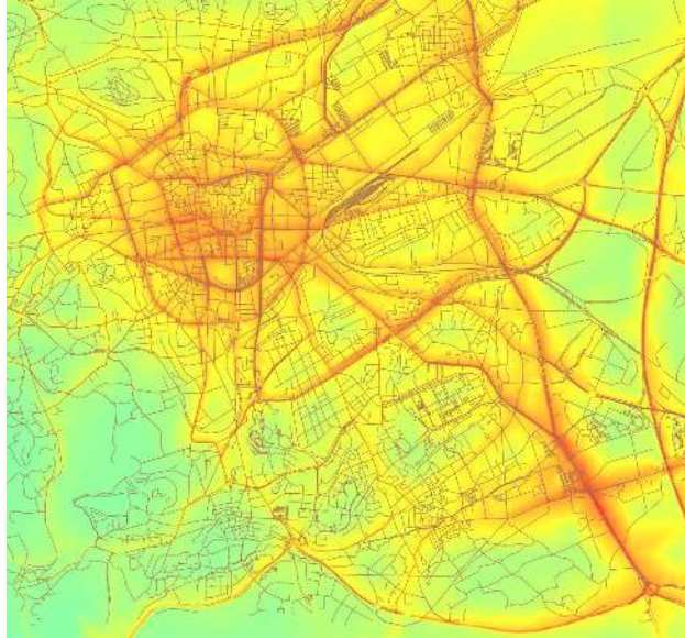
Figure 1: Hourly map of concentrations of nitrogen dioxide as computed by an urban air quality model over Clermont-Ferrand (France). The objective of the post-doctoral position is to quantify the uncertainties associated with such maps.
