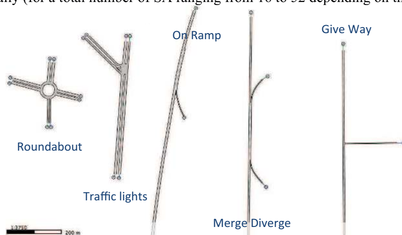
Figure 1. Layout of the five test networks. As the layout changes, the effect of the different parameters on the outputs changes as well.
