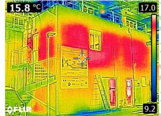
Building surface temperature obtained with an infrared camera in the Equipment Sense-City
