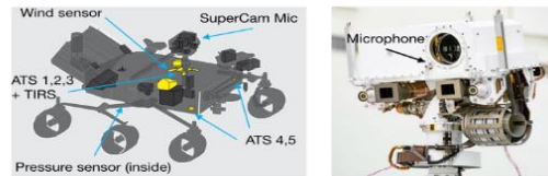
Figure 1. (Left) Diagram of the Perseverance rover with the locations of instruments used highlighted. (Right) Picture of the mast head housing the SuperCam instrument with the microphone location indicated. Credits NASA/JPL-Caltech for the right image, adapted from Maurice et al. (2021), Mimoun et al. (2023).
