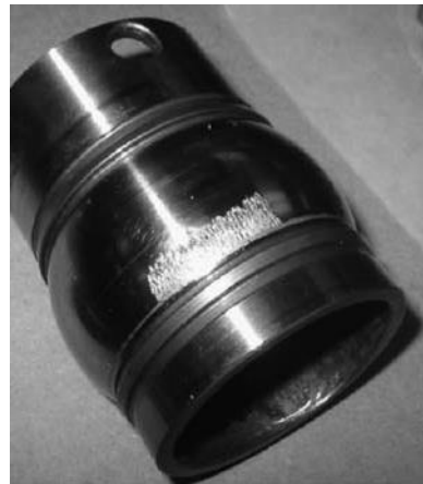
State 4: Severe degradation
